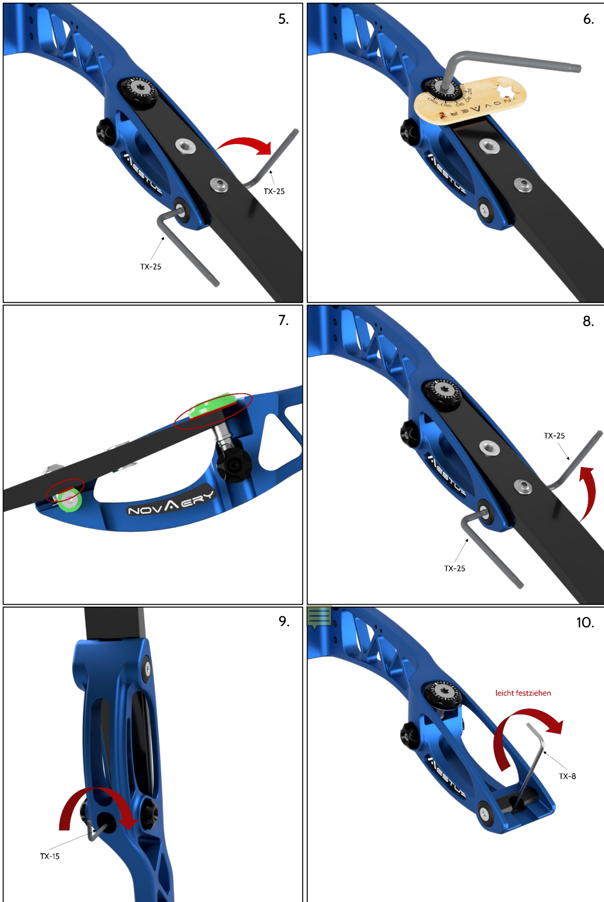
Figure 9: Adjusting the Tiller Screw
